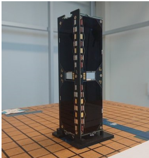
Figure 2.7: Delfi-PQ PocketQube by TU Delft [10].
