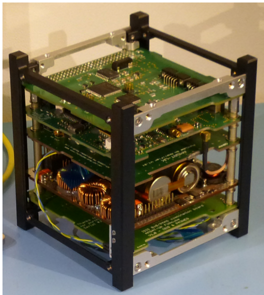
Figure 4.31: Engineering model of FUNcube-1 without the outer panels attached [61].
