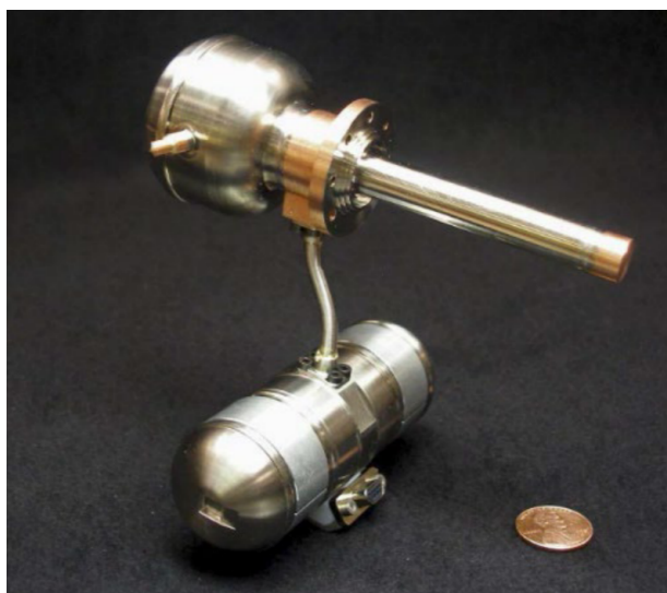
Figure A.13: Micro-cryocooler by Lockheed Martin [16].
