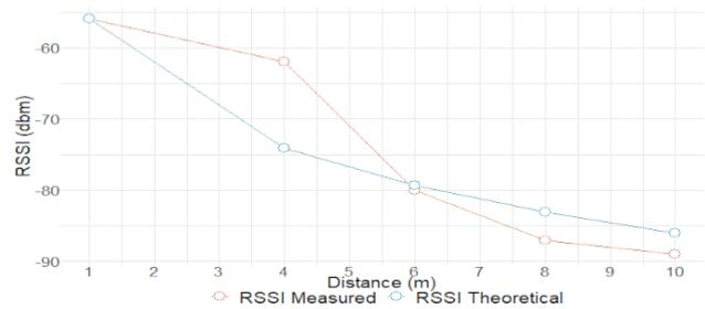
Figure 6. RSSI signal behavior in an obstacle scenario
