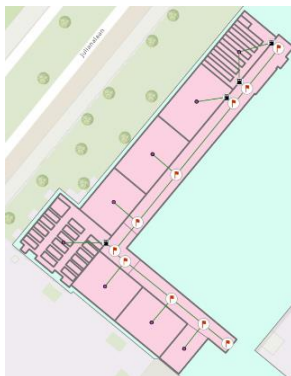
Fig. 4. ArcGIS Indoors topological relationship between rooms of the West Wing of TU Delft faculty of Architecture
