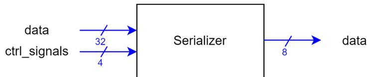
Figure 5-2: Designed Serializer block.
