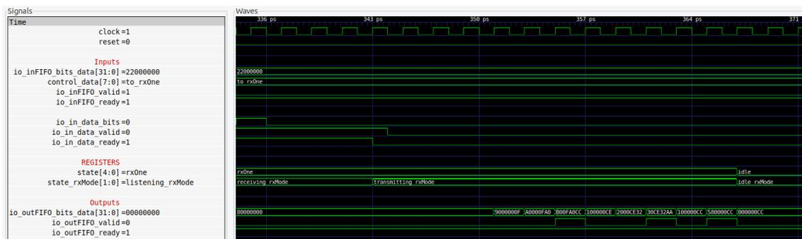
Figure D-5: End of the reception of a packet in simple Rx mode.
