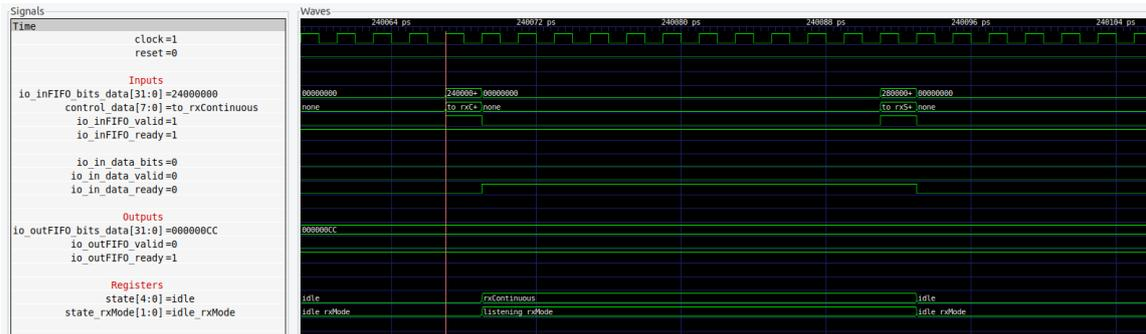
Figure D-16: Rx continuous mode and rxStop command SoC simulation.
