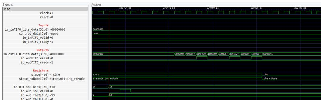
Figure D-17: Single bit error correction SoC simulation.
