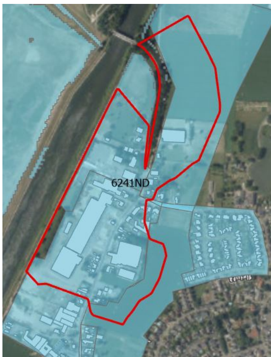
Figure A.16: This business area has much lower reported damages than was reported on average in comparison with the GFRT. This indicates that very little flooding may have actually occurred here.
