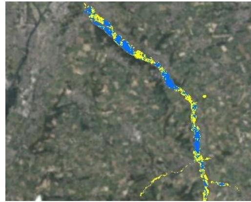
Figure 5.1: Visualisation of the manually inserted 0,5m inundation cells at the middle Geul section. Yellow indicates grid cells with 0,5m whereas blue is the underlain flood extent map.
