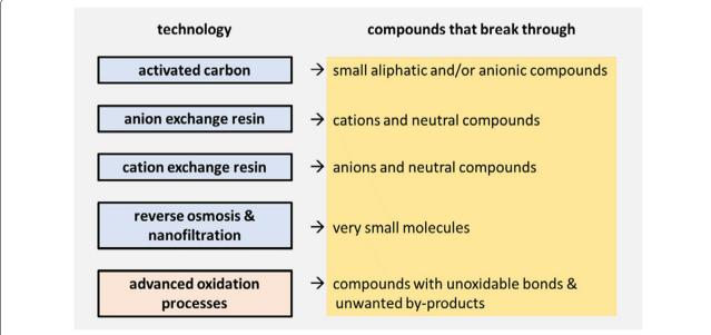
Fig. 4 Water treatment technologies (left column) and the organic compound groups that cannot be removed by the respective method and/or can survive treatment (right column)
