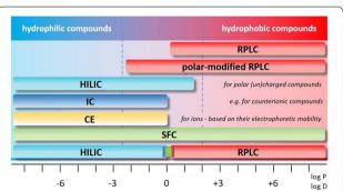
**Fig. 2** Polarity scheme for chromatographic (electrophoretic) separation techniques (like reversed-phase liquid chromatography (RPLC), hydrophilic interaction liquid chromatography (HILIC), ion chromatography (IC), capillary electrophoresis (CE) and supercritical fluid chromatography (SFC)) based on log D<sub>ow</sub> values (at several pH values) of separable molecules and molecule characteristics, [48] adapted with polarity extended chromatography [49]
