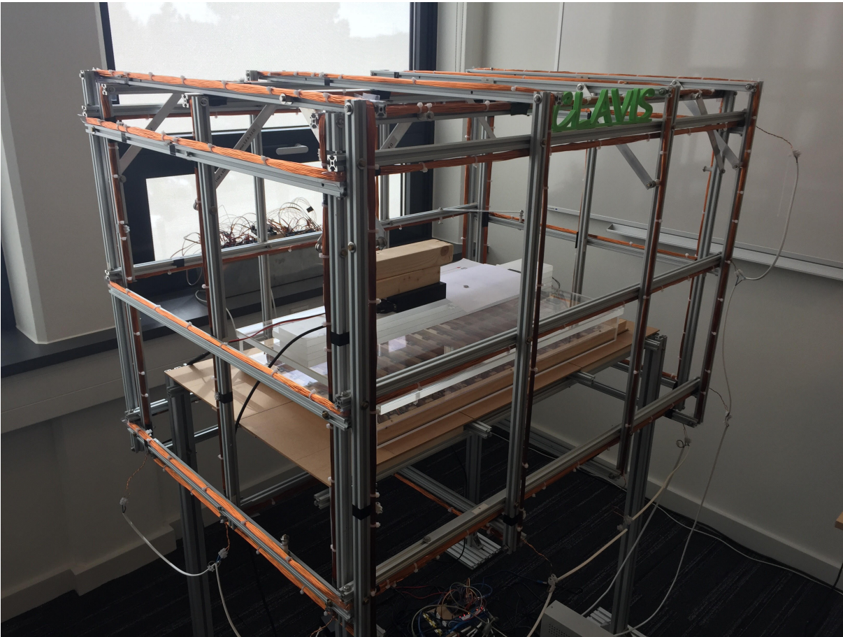
Figure B.5: Aluminium frame with coils in x , y and z -directions.
