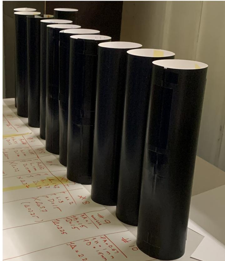
**Figure 4.3:** The cylinders sleeves after being taped into the a round shape to fit over the PVC pipe base.
