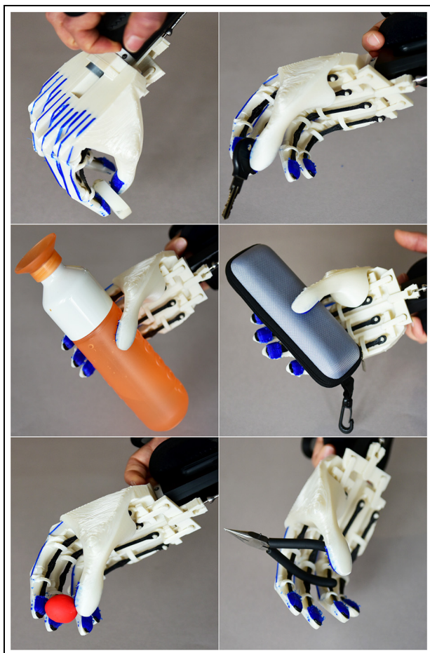
Figure 5. The grasping patterns. (top left and right) Pinch grasping, (middle left and right) power grasping, (bottom left and right) and tripod grasping.
