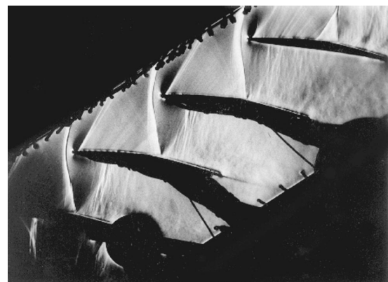
Figure 1.2: Oblique shocks in a compressor cascade. From (Weber et al., 2002).
