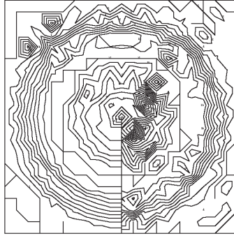
Figure 7.3: Equi-concentration lines for rotating cone problem computed by SGA.
