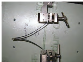
Figure 6.41 Typical example of a peel test on one of the ABS samples tested according to ASTM D1867.
