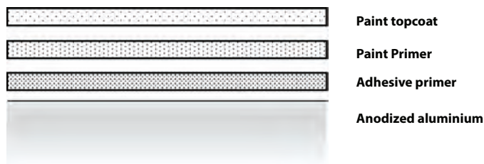
Figure 6.21 Schematic representation of chromic acid anodized aluminium with the adhesive primer and paint layers (not to scale).
