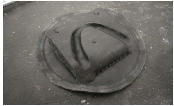
Figure 93. Multi-stage thermoforming on an aligned mould results in much gentler deformations.
