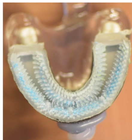
Figure 38. Single membrane actuation as used in the standard mouthpiece.
