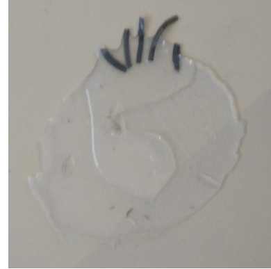
Figure 49. FDM bristles between silicone layers.
