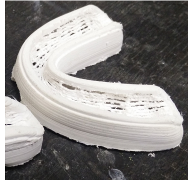
Figure 96. Disconnected edges improve flexibility.
