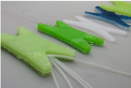
Figure 42. Simple adhered soft robot (Wu, 2018)
