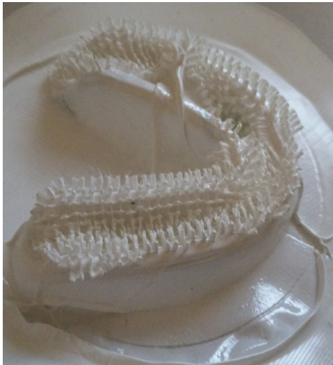
Figure 71. Frame/sheet assembly after being deformed
