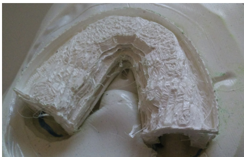
Figure 72. Deformed frame with bristle sheet
