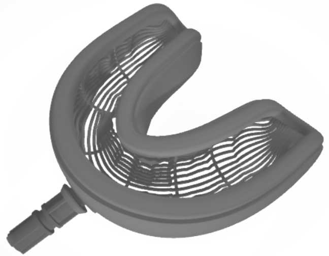
Figure 99. Mesh built from 'wires' parallel to the dental arch
