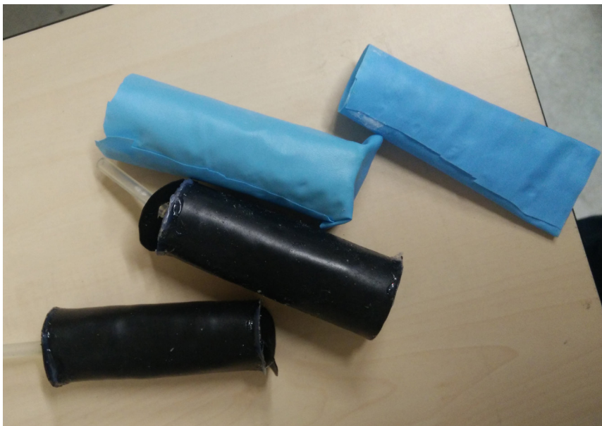
Figure 51. From bottom left to upper right: Dual layer .8mm, mesh + .8mm, mesh + .4mm, and dual layer .4mm TPE tests
