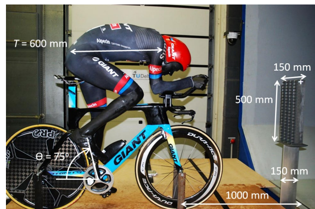
Fig. 2 Wind tunnel model and PIV seeding system
