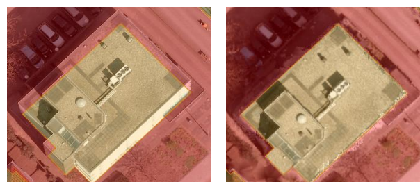
a. Building misalignment between the map (yellow) and image b. A matched building in the map and image
