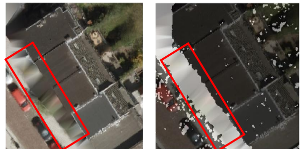
Figure 5. The blurred pixels shows the occluded area (inside the red rectangle)
