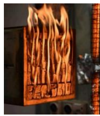
Figure 5-8: Flaming of uncoating test sample (Lucherini et al., 2019)
