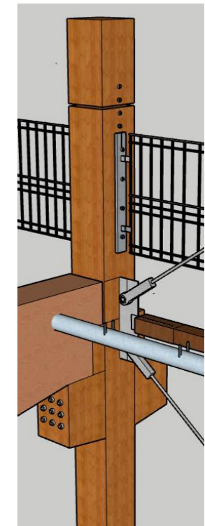
Figure I-20: 3D view edge column without floor system
