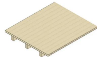
Figure 6-18: Open CLT rib floor Stora Enso ( Rib Panels, n.d. )
