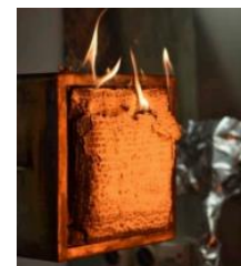
Figure 5-9: Flaming coated test sample (Lucherini et al., 2019)
