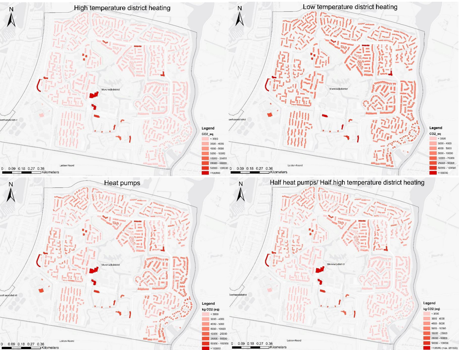
Figure 23 Four maps that presents the kilograms of CO2 (eq) for the required materials for all four scenarios in the Merenwijk on residential building level
