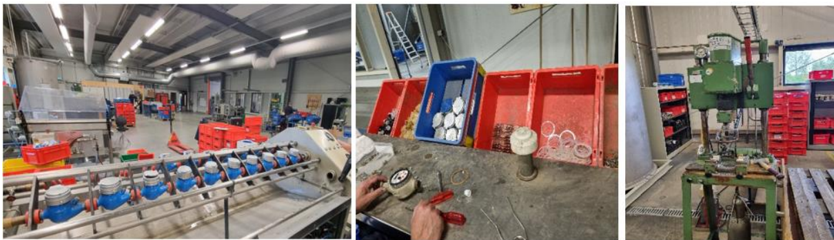
Figure 33: Water meter refurbishment process (inferential M100 model)
