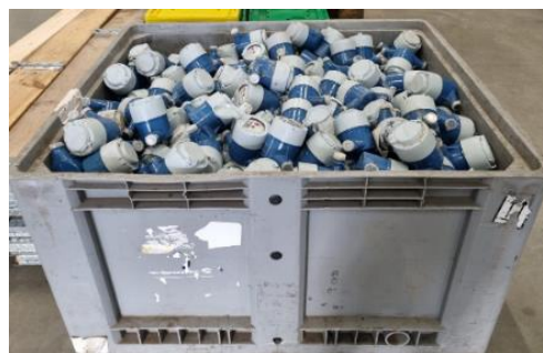
Figure 35: Example of bins for EoL water meter collection at DWUs
