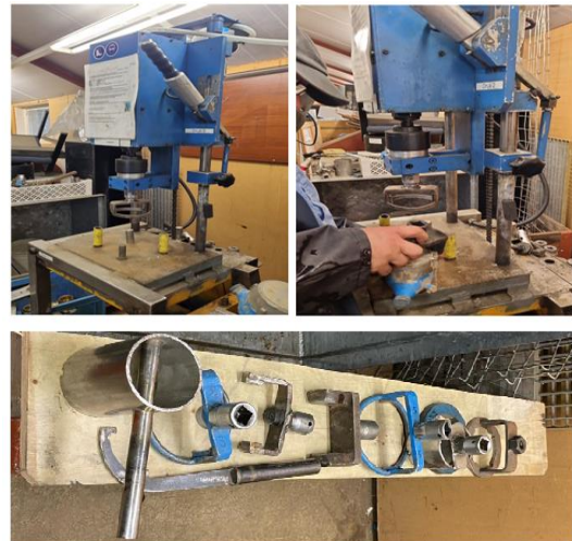
Figure 9: Mechanical aids and clamps for the disassembly of various water meter designs. Source: WoW
