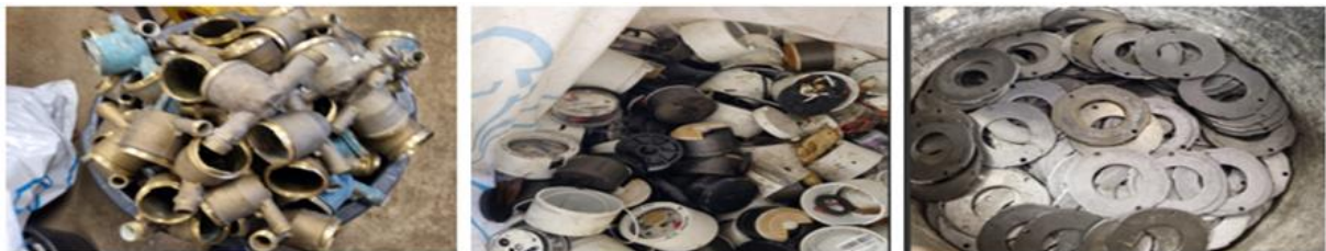
Figure 10: Sorting of water meter materials: Brass (left), plastics (middle), stainless steel (right). Source: WoW
