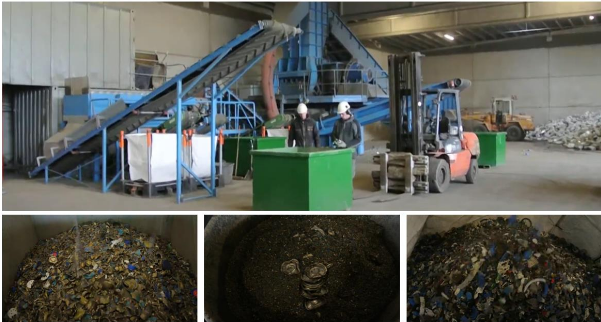
Figure 11: A typical industrial shredder and automated sorting system featuring three distinct output streams arranged from bottom left to right: brass, glass and non-ferrous metals, and plastics. Source: Metal Recycling (2014)
