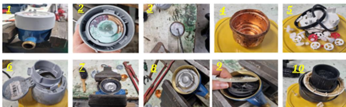
Figure 31: Images of the disassembly process for the Elster V200 Water Meter
