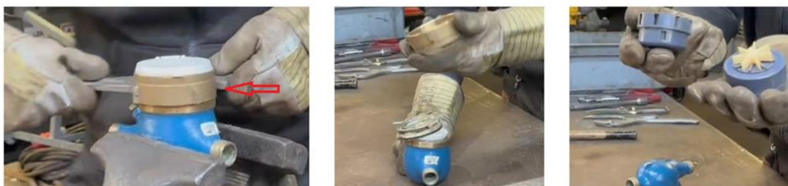
Figure 8: Images from the disassembly process of the M100 meters. Red arrow indicating the registry cover. Source: RC II
