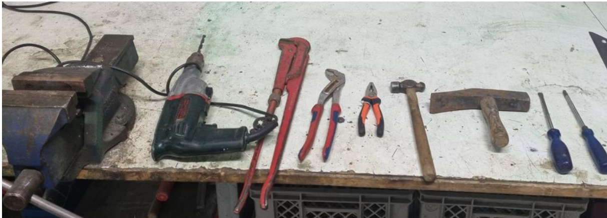
Figure 28: Tools used for the disassembly method. From left to right: Vise clamp, electric drill, multiple pliers, two sets of hammers and a flat and Philips head screwdriver.
