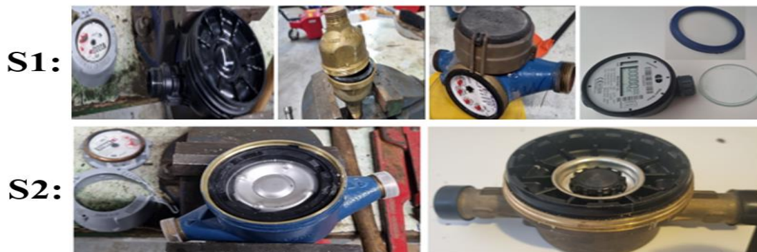
Figure 30: Dismantled meters. Left to right S1: Elster V200P, V100, M100, Kamstrup Multical 21. S2: Elster V200, Itron Flodis
