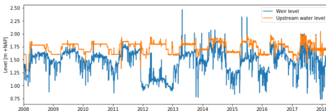
Figure 3-4, weir level and upstream water level at Buren between January 2008 – April 2018.
