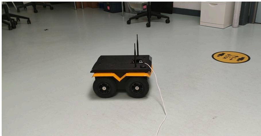
Figure 1.2: The Clearpath Jackal robot in the lab (for scale), tethered to a computer running an active inference node
