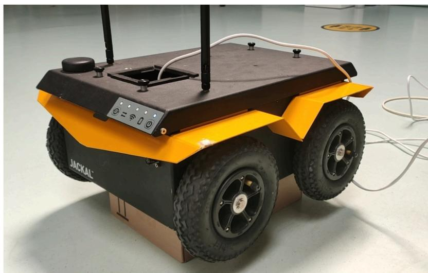
Figure 3.3: A photo of the Jackal robot for the the on-box experiments, where the wheels are suspended in the air
