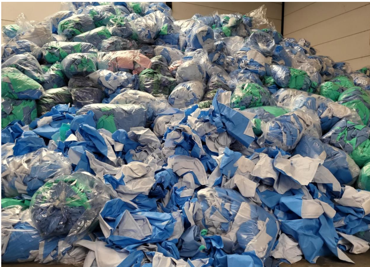
Figure 6. Urban mined polypropylene from Maastad Hospital, used to melt into polypropylene granulate, which is used to injection mold dog bones and other products. Photo by Bart van Straten.
