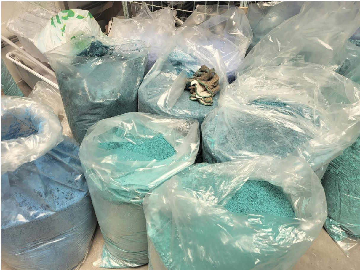
Urban mined Polypropylene blue wrap, ground after melting. Photo by Bart van Straten.
