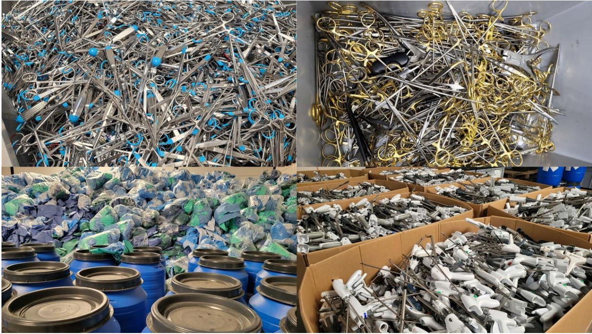
Examples of urban mined waste consisting of stainless steel, polypropylene blue wrap and complex surgical devices with a variety of valuable components and materials. Photos by Jeronimus van Pelt.
