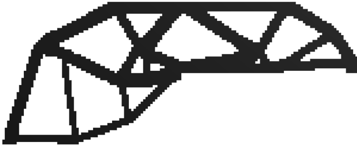
Figure 3.4: The binary image based on the TO result.
