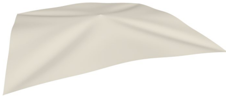
Fig. 13 Deformed surface from the benchmark presented in Fig. 12. The result is the last solution from the adaptive meshing routine with deformation norm goal-functional of which the results are presented in Fig. 14
