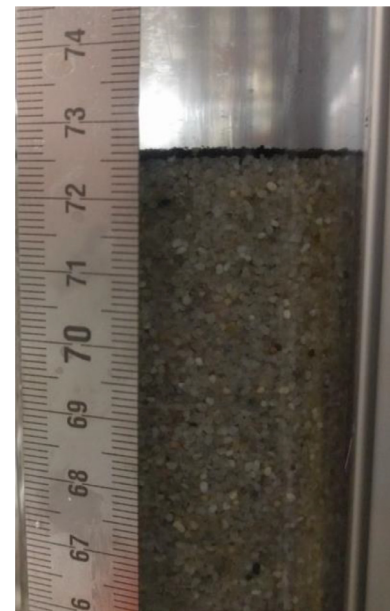
Fig. 13. Fixed bed setting after t=5 [min] ETSW.
