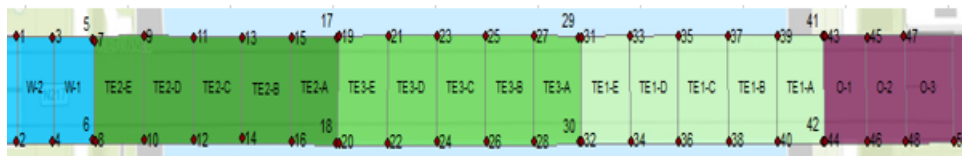
Figure 5.2: Arrangement of settlement measuring points
