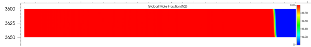
Figure 26: Mixing zone between nitrogen and residual methane showing smaller mixing front. 100% Concentration of nitrogen is shown in red. 100% Concentration of residual methane in blue.
