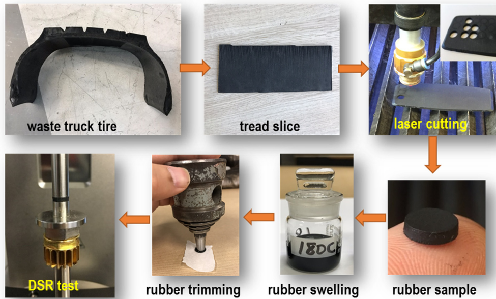
Fig. 2. Preparation of cylindrical dry rubber and swollen rubber samples.
