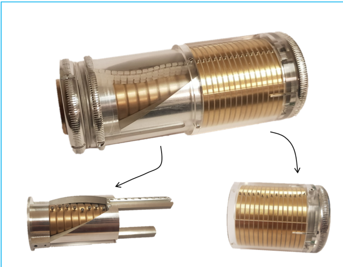
Figure 6.1: Pictures of the machined prototype. The upper picture is the complete prototype. The picture in the left corner shows the 8 memory rings, contained within the translational motion mechanism. In the bottom right, the output is shown: the reading rings and Teflon frame are contained in a perspex casing.
