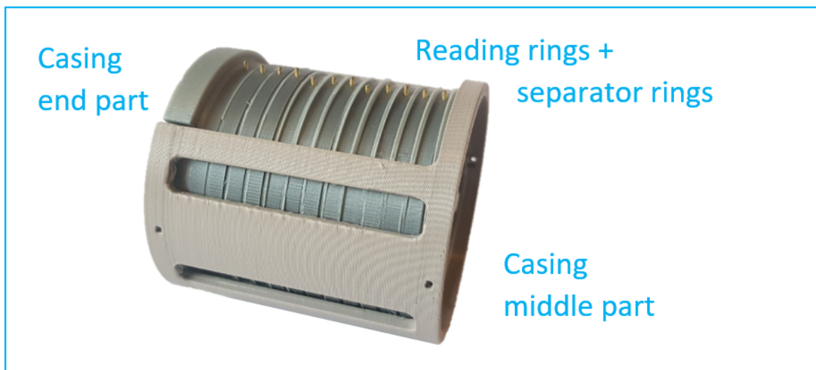
Figure E.30: Picture of the reading rings in their frame from the 3D printed prototype
