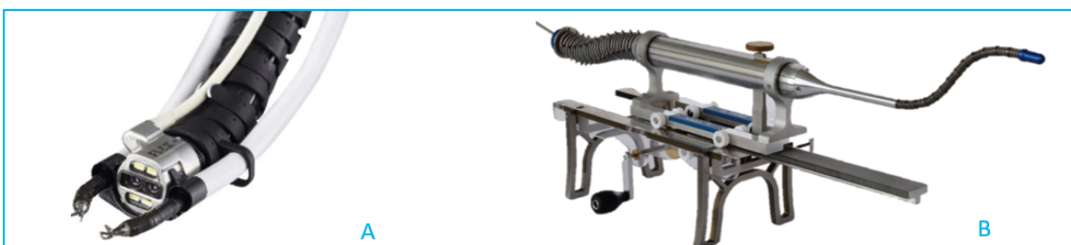
Figure 1.3: The Flex system (Medrobotics, Raynham, MA, USA) and MemoFlex I (BITE, Delft, The Netherlands). Figure A is the Flex system. Inside the black tube, two concentric tubes can rotate and translate with respect to each other. It is an alternating telescoping robot, that is designed for medical applications. Figure B shows the MemoFlex I. It is a shape-shifting mechanism that is fully mechanically controlled with cables. The images are adapted from Medrobotics Corp. [9] and BITE group [6].
