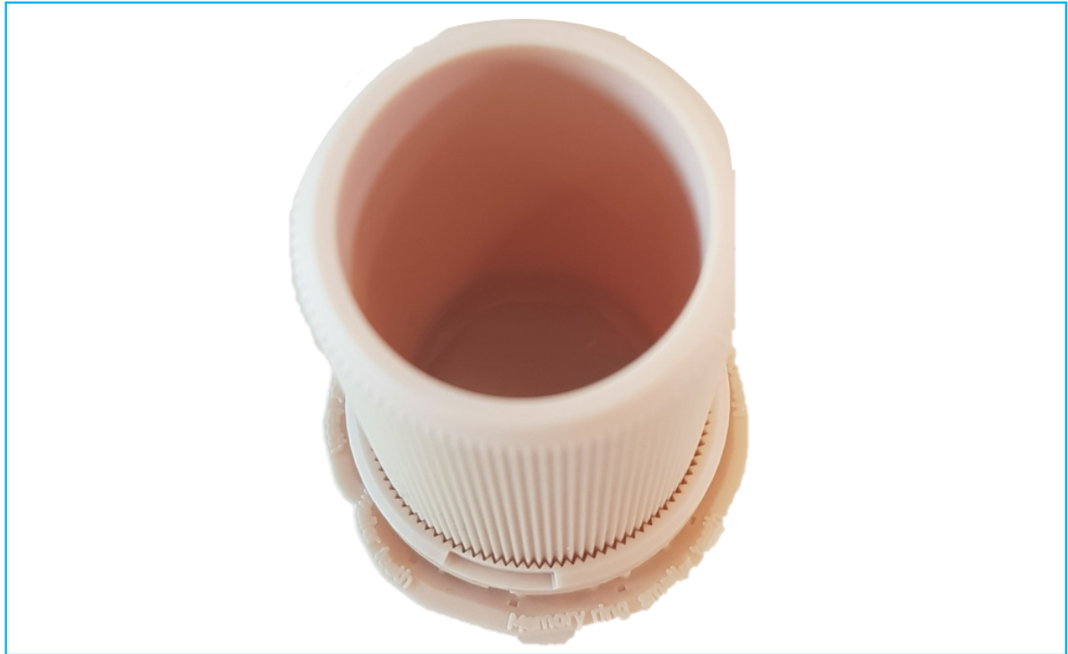
Figure E.23: 3D printed shaft and memory ring version 3
