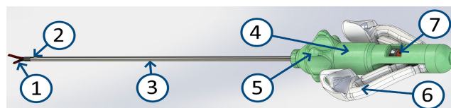
FIGURE 6. Compliant instrument design overview, with grasper tip (1), tip locking mechanism (2), shaft (3), balancing mechanism housing (4), rotating interface (5), handle (6) and push pull rod locking (7). Note that the used colors do not represent the final prototype.
