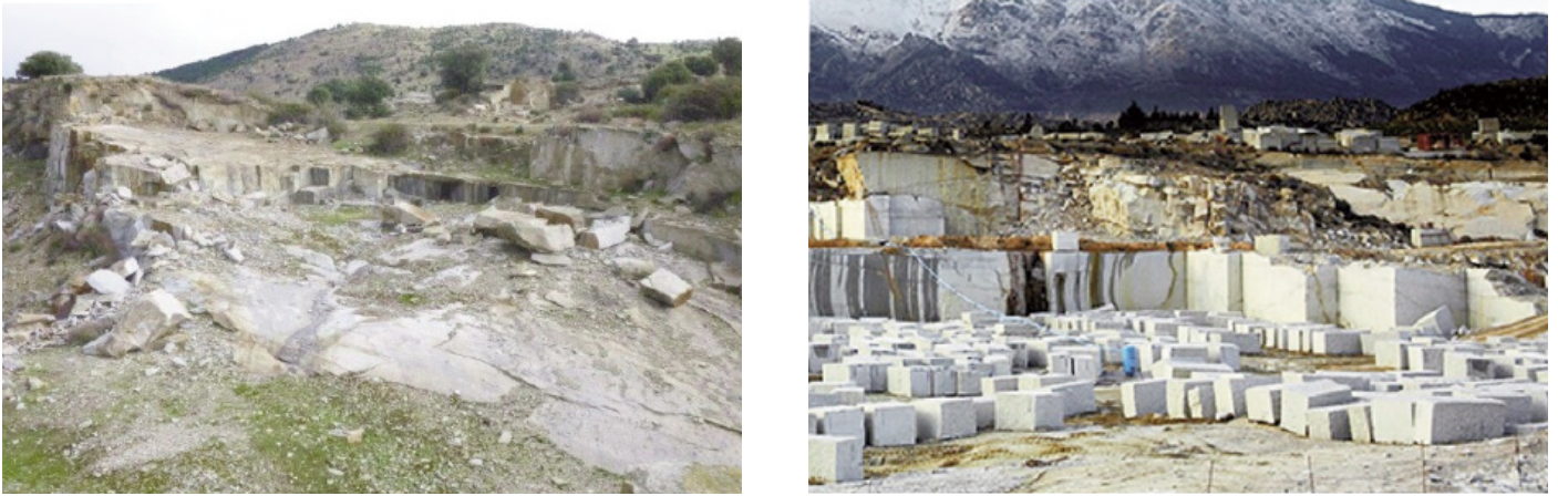
Figure 8 - Differences in past and present extractive processes: overgrown landscape of historic outcrop quarry in Alpedrete and invasive quarry operation in La Cabrera (left to right) (Freire-Lista 2016).
