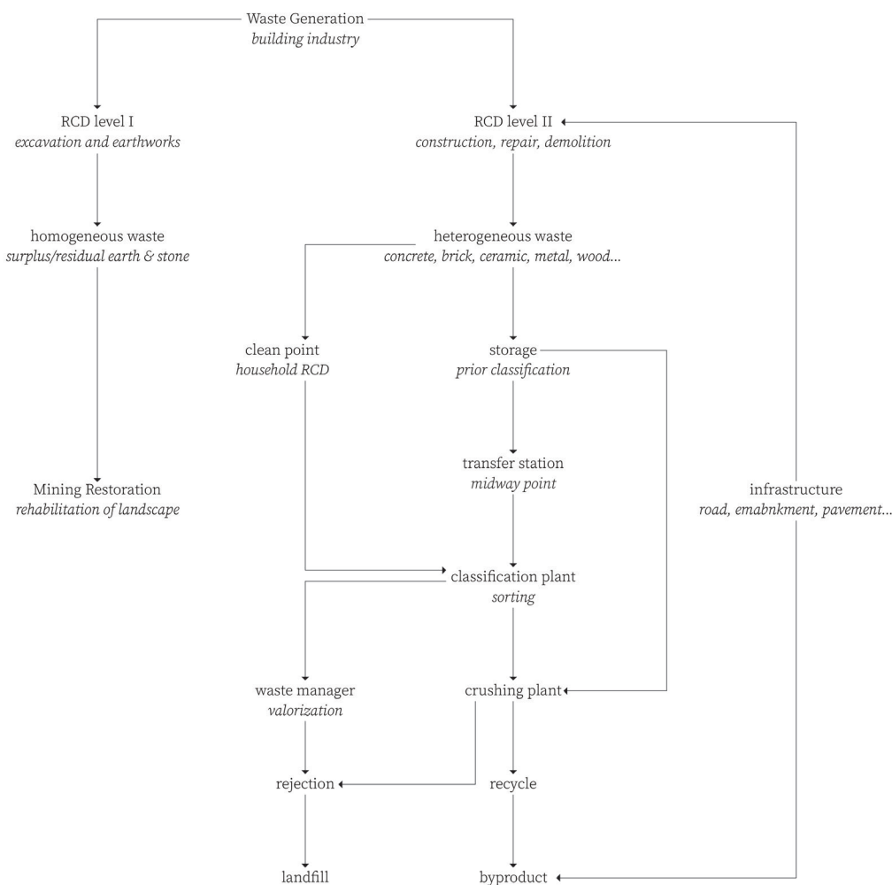
Figure 11 - diagram of Madrid's waste processing system from collection to byproduct for recycling (author's diagram)
