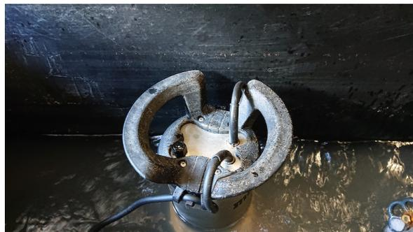
**Figure C-8:** Water pump. The pumps are located inside water basin under the testbed.
