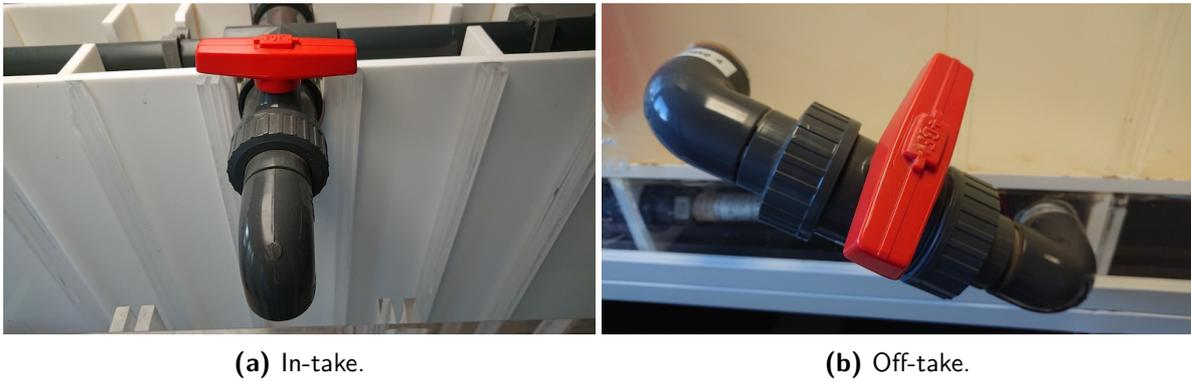
**Figure C-5:** In- and off-takes to simulate disturbances. The in- and off-takes for  $pool_1$  to  $pool_3$  are controlled by hand.
