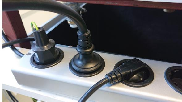
**Figure C-7:** Power supply for the testbed. There are no switches for the pumps, so they are operated by plugging them in. The plug on the left is used to connect the testbed to the ground.
