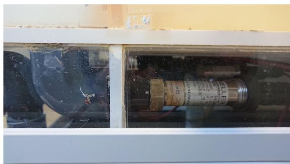
**Figure C-9:** Pressure sensor. The sensors are located under the pools.
