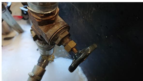
**Figure C-4:** Main valve. The main valve leads to  $pool_0$  and has to be controlled by hand.
