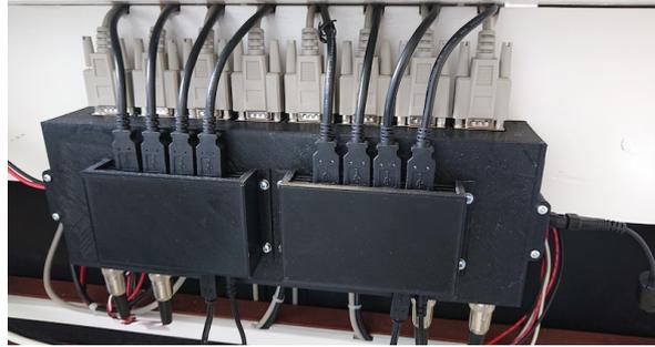
**Figure C-10:** Powered usb-hubs. The Fireflies are connected to powered usb-hubs in the following order (left to right): FF4, FF3, FF6, FF8, FF5, FF7, FF2, FF1.
