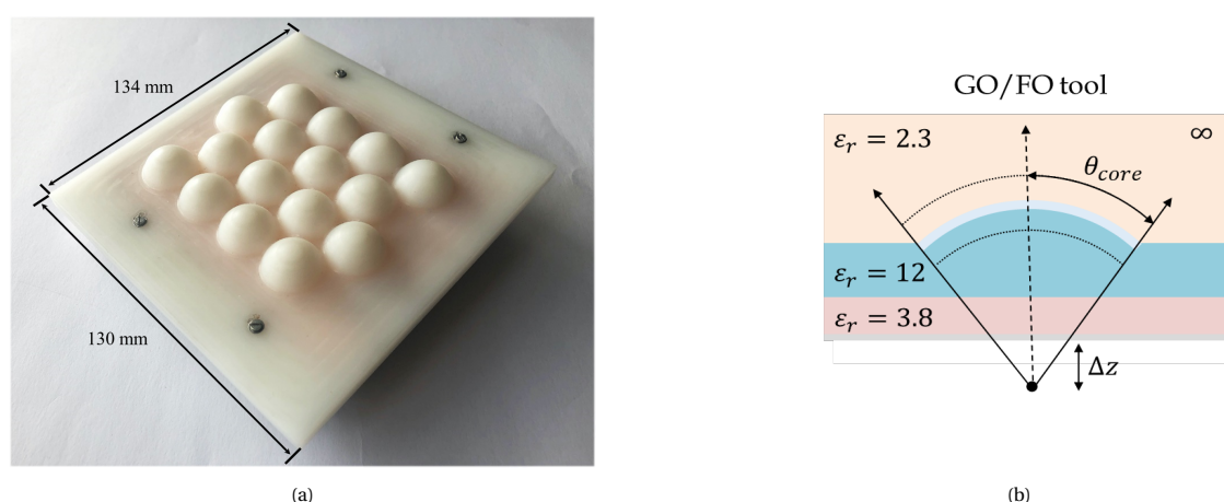
Figure 1.1: Applications using small lenses in (a) Phased array using 2\lambda_0 lens as elements [1] and (b) Core-shell lens design for fly eyes applications [2]
