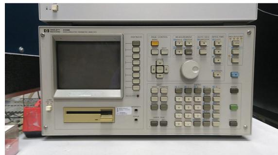
(b) The HP4145B parameter analyser used to set the bias voltages and read the drain current.
