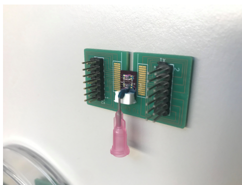
Figure 11.1: Thruster on the PCB with pressure sensor from Prof Henk van Zeijl at EWI
