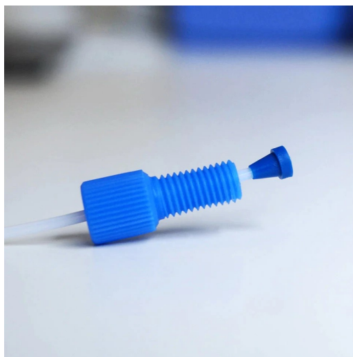
Figure 6.27: 1/4-28 fittings connector for the connection with microfluidic components
