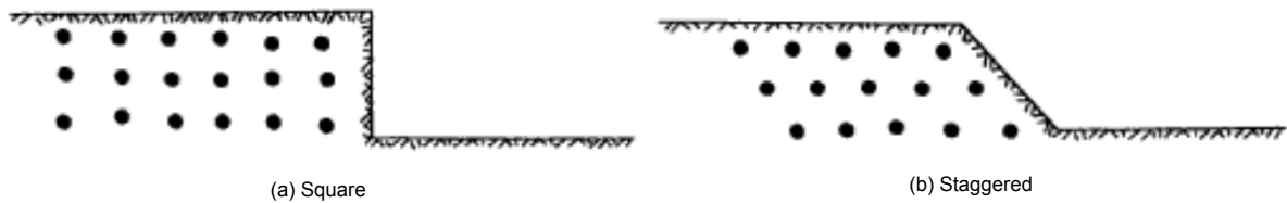
Figure 2.2: Square and staggered blast pattern layout [4].
