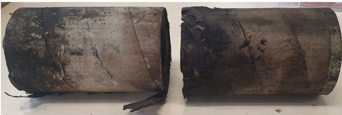
Figure 5.8: Grains after the forward closure ruptured and a rapid depressurisation caused them to extinguish.
