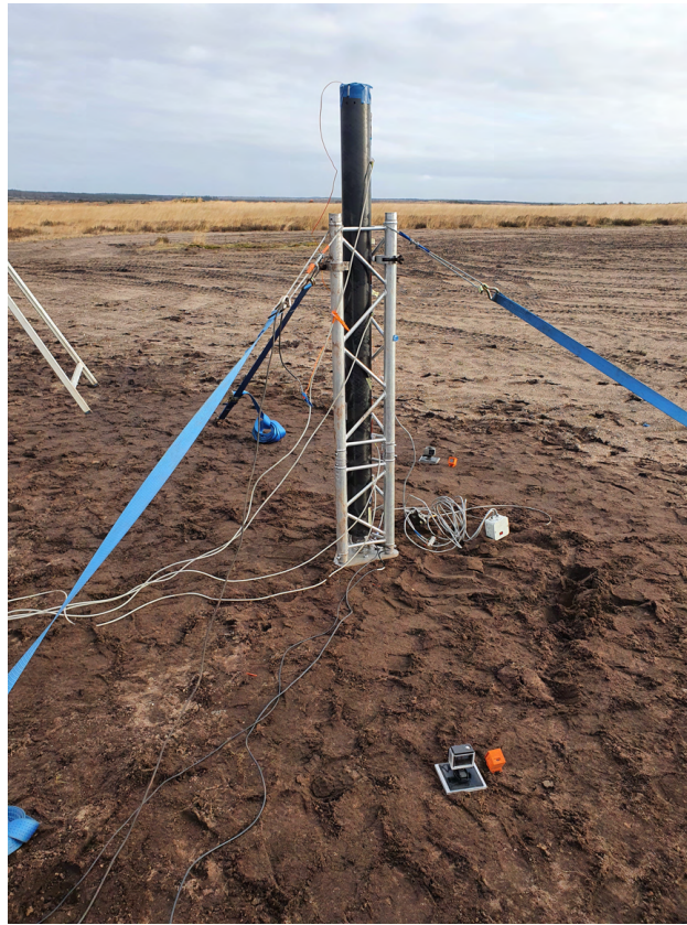
Figure 3.15: Overview of the test setup showing the cables that run from the strain gauges to the data acquisition system.
