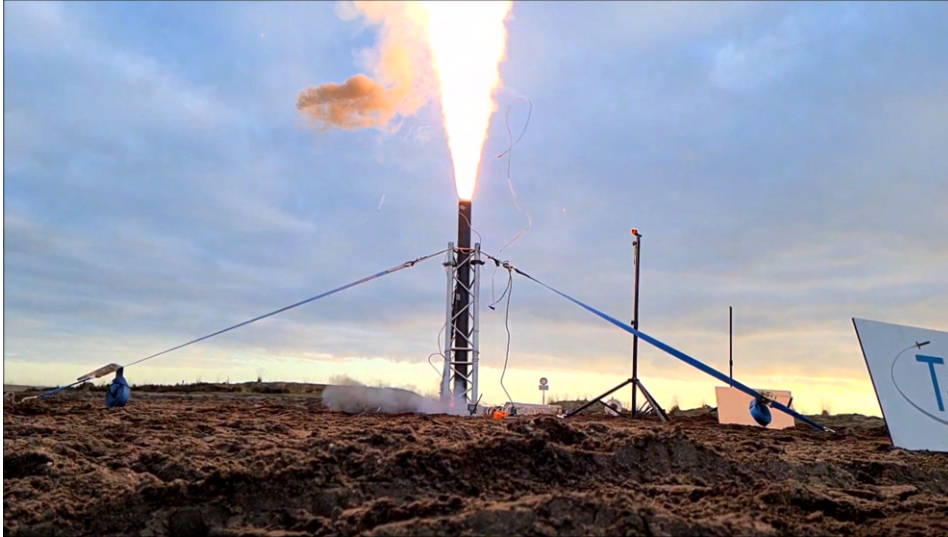
Figure 5.7: Overview of the setup during hot fire, note the smoke on the side of the forward closure causing the sudden depressurisation.
