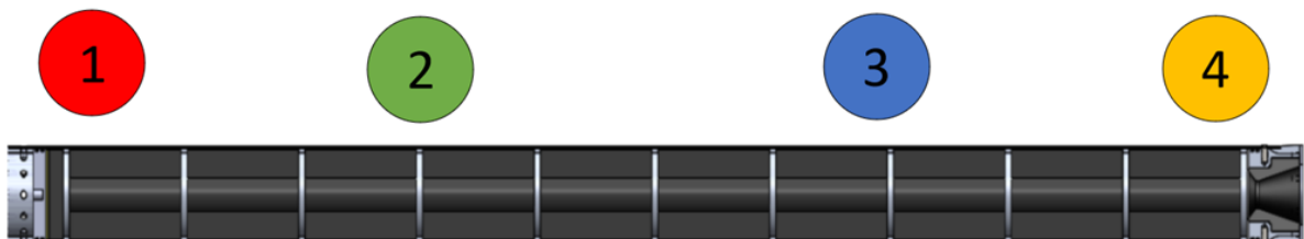
Figure 3.14: Schematic of the placement of the sensors, note that all locations are chosen next to spacing in between the propellant segments or grains.
