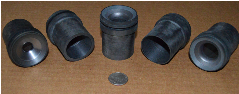
Figure 2.5: Small single-use nozzles made from linen phenolic with a graphite throat give an idea of what a nozzle of a (smaller) solid rocket motor can look like. [14]
