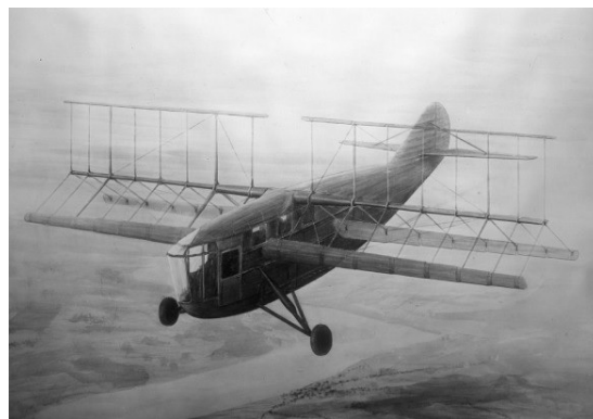
Figure 3.31: Rohrbach cyclogyro (1933), from MSW [64]
