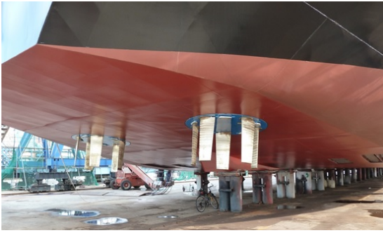
Figure 3.32: Voith-Schneider propellers on a ferry, from Fornas et al. [35]
