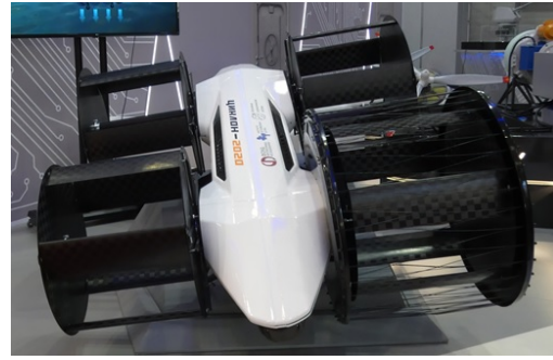
Figure 3.33: Quadcopter drone with cyclorotors, from Wikimedia [82]
