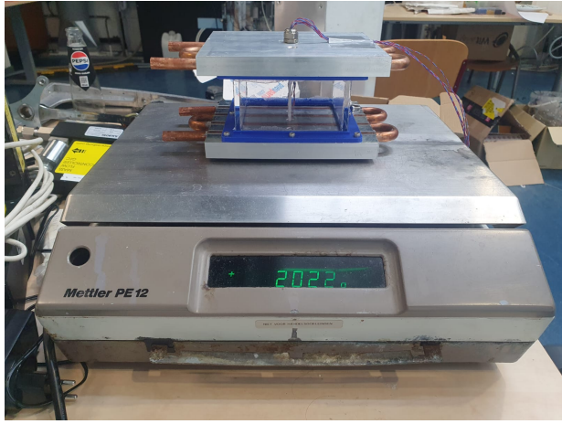
(a) Plexiglass enclosure without PCM.
