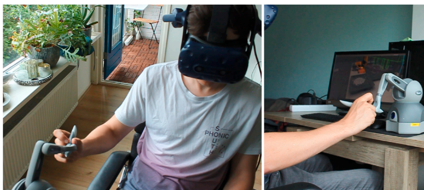
FIGURE 1 The system used in the experiment setup consisted of the stylus of the Touch Haptic Device and HTC Vive Head-Mounted Display.
