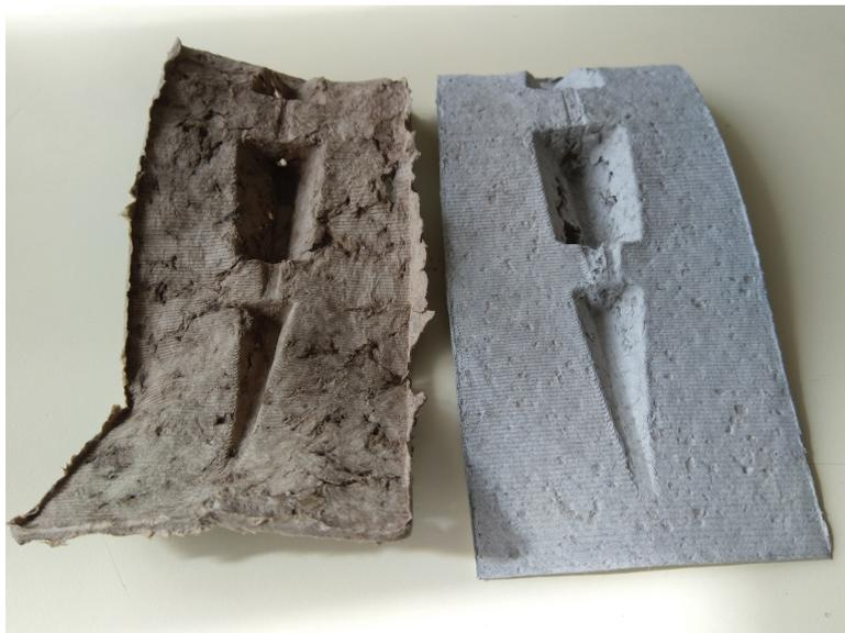
Figure 11.4: Paper pulp wing section samples, first experiment on the left, second one on the right.
