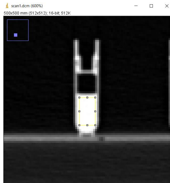
Figure 21: ROI selection with ImageJ for HU calculation of each commercial sample of different concentration
