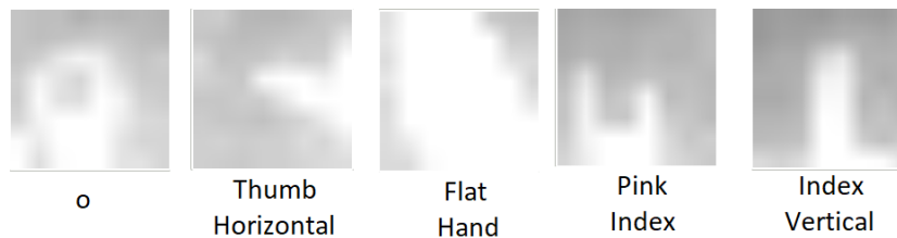
Figure 8.1: Examples of 8 by 8 images made with the AMG Grid Eye, the ".png" format smoothens the pixels out to make it look more natural.
