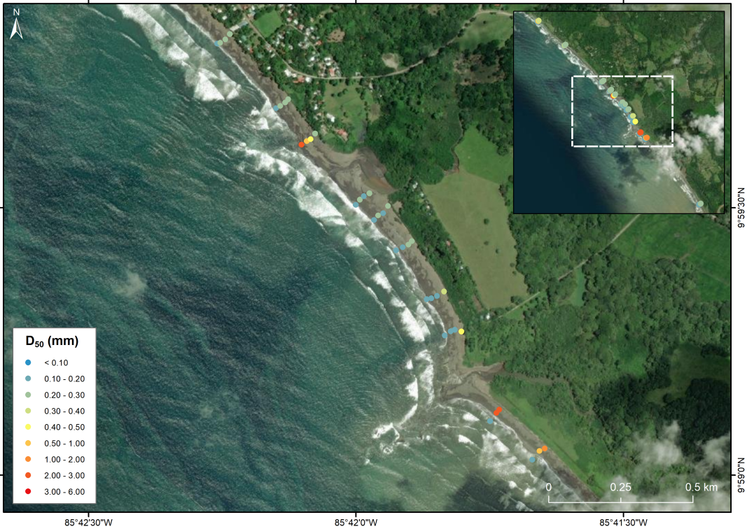
Figure 3.11: D_{50} of samples in dry season, with a focus on Main Nesting Beach
