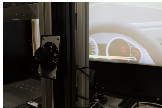
Figure 6.2: The turning knob with which participants can indicate the perceived motion mismatch. The rating bar on the background shows the current rating.
