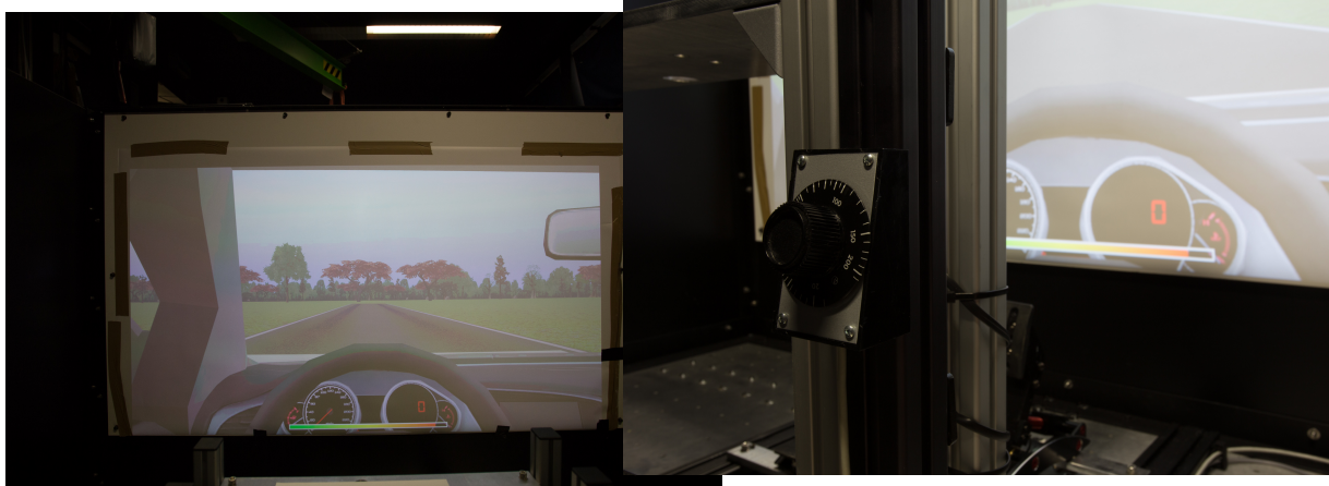
Figure 4.3: The turning knob with which participants can indicate the perceived motion mismatch. The rating bar on the background shows the current rating.
