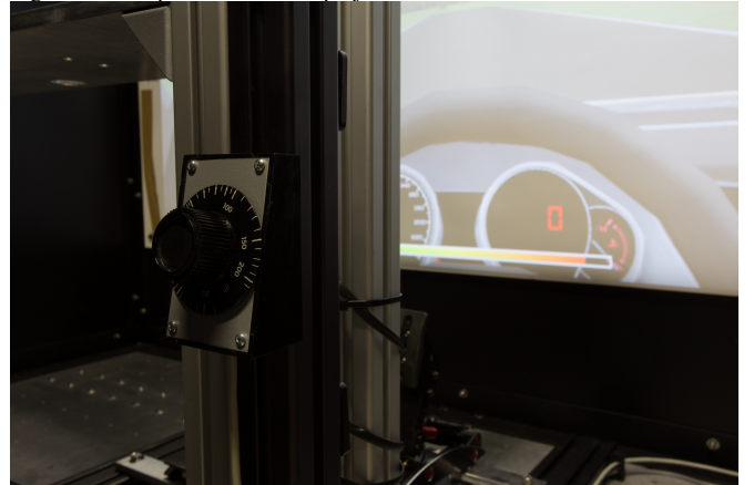
Fig. 10. The turning knob with which participants provided their continuous rating. The rating bar on the screen shows the current rating.
