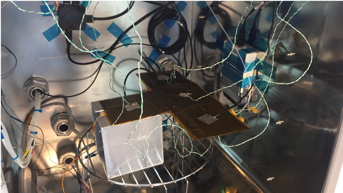
Figure E.4: The DRW prototype in the test set-up inside the vacuum oven. The green white wires are the thermocouples.
