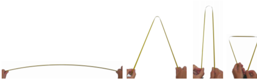
Figure 3.3: Folding of a tape spring [26].
