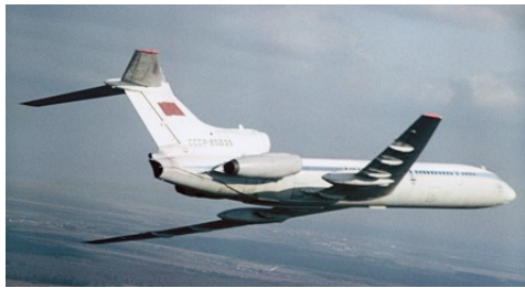
Figure 2.3: Soviet experimental Tupolev-155, powered partially on LH_2 . [41]
