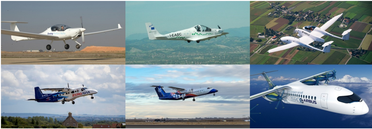
Figure 2.6: Hydrogen fuel cell propulsion demonstrators and concepts: Boeing first ever manned fuel cell aircraft, ENFICA-FC, H2FLY HY4, ZeroAvia Do228, Universal Hydrogen, Airbus. Reproduced from [5, 6, 7, 8, 9, 11]
