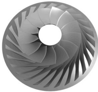
Figure 3.16: Transonic impeller design by Zangeneh et al. [165].
