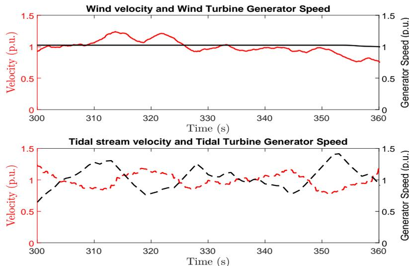
**Figure 17.** Comparison of generator speed fluctuations in a 10 MW wind turbine and a 110 kW tidal turbine.
