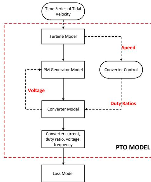
Figure 12. Internal structure of the PTO model.
