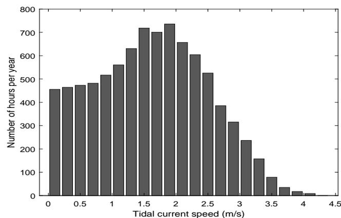
Figure 3. Tidal velocity distribution at EMEC site, Orkney [31].
