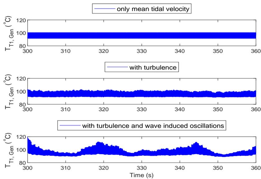
**Figure 19.** Temperature of the Generator Side Converter insulated gate bipolar transistor (IGBT) (T1) as a function of the fluctuations in the tidal stream velocity.
