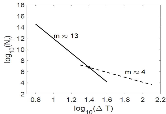
**Figure 13.** Number of cycles to failure are presented as a function of temperature cycling for a constant mean junction temperature.
