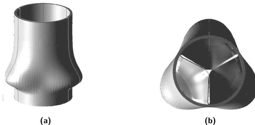
Figure 1.3: Representation of the AR. In (a), lateral view which highlights the bulged shape of the sinuses. In (b), top view shows the interconnections between sinuses and leaflets. Pictures are taken from [34].
