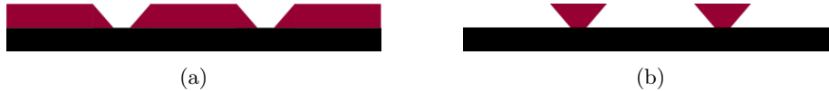
Figure 5.2: The resist pattern left behind due to overexposure of a (a) positive and (b) negative resist using the same mask pattern as in Fig. 5.1a.
