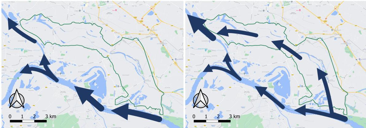
Figure 6.2: Altering the water distribution at the Pannerdensche Kop: with flow through the Rijnstrangen more water can be lead to the Lower Rhine (northward from the bifurcation), instead of the Waal (southward from the bifurcation).
