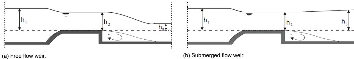
Figure 4.2: The two weir types, both adapted from Bezuyen et al. (2012).
