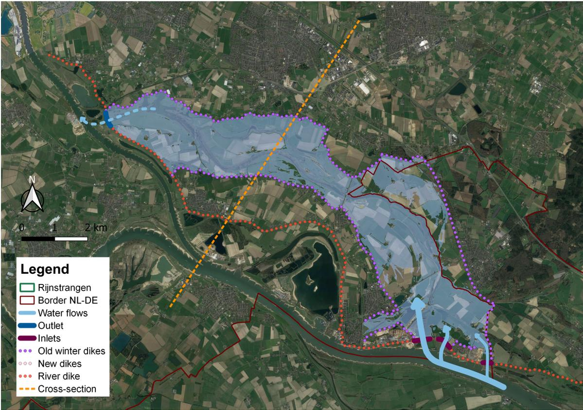
Figure 3.1: Concept of the Rijnstrangen as retention area. Here the water level is set to 13.0 m +NAP as an example. The cross-section is referred to in Figure 3.4.
