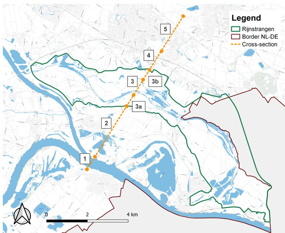
Figure 4.3: Map of cross-section chosen for the groundwater calculations. This cross-section corresponds with B - B\* of Figure 2.8 and with the cross-section in Figure 3.1. It is assumed that groundwater flow along this cross-section is representative for the entire Rijnstrangen. The numbers indicate the different sections as used for the calculation of the groundwater flow.
