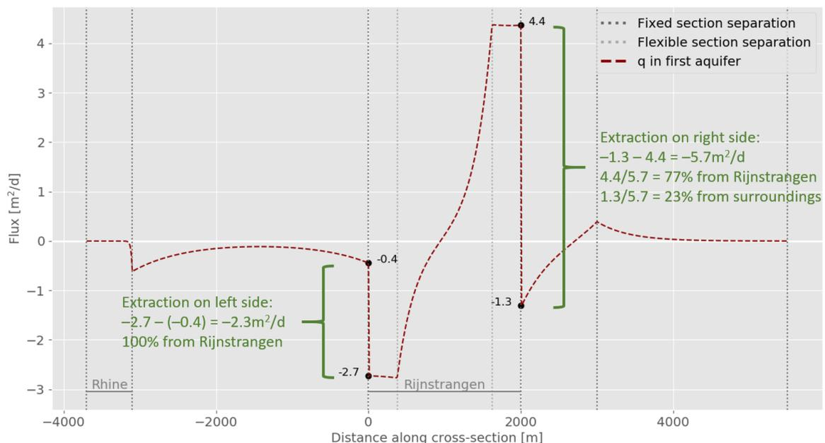
Figure 4.16: Example of a groundwater flux plot along the cross-section used for the groundwater calculations. This data can be used to analyse the groundwater exchange between the Rijnstrangen, the surrounding region and the extraction wells. A positive value indicates a groundwater flow in northward direction, a negative value indicates a southward groundwater flow.
