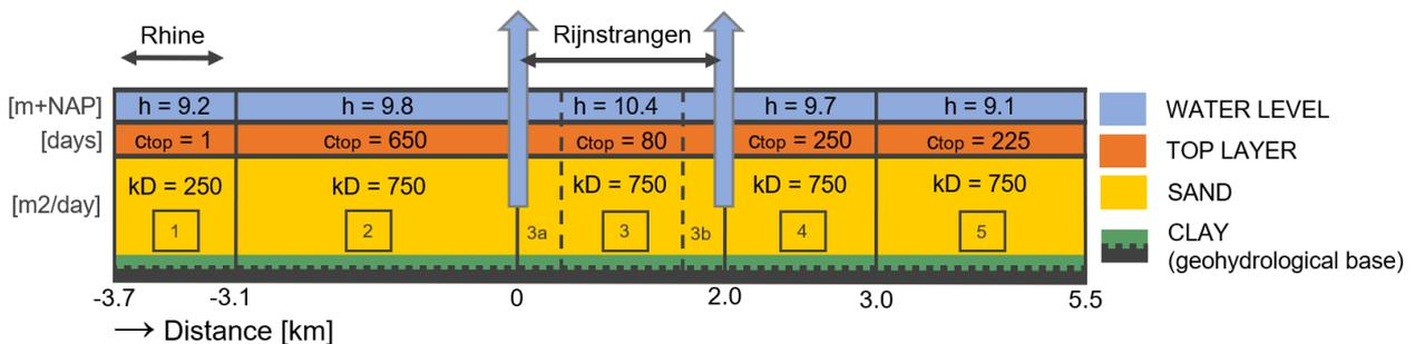
Figure 4.6: Schematization of the geohydrological situation used for the groundwater calculations. The values in this figure together form the input vectors and matrices. Sections 3a, 3 and 3b have a variable width. The hydraulic resistance of the top layer under the Rhine is very low, here the Rhine water stands in direct connection to the groundwater.
