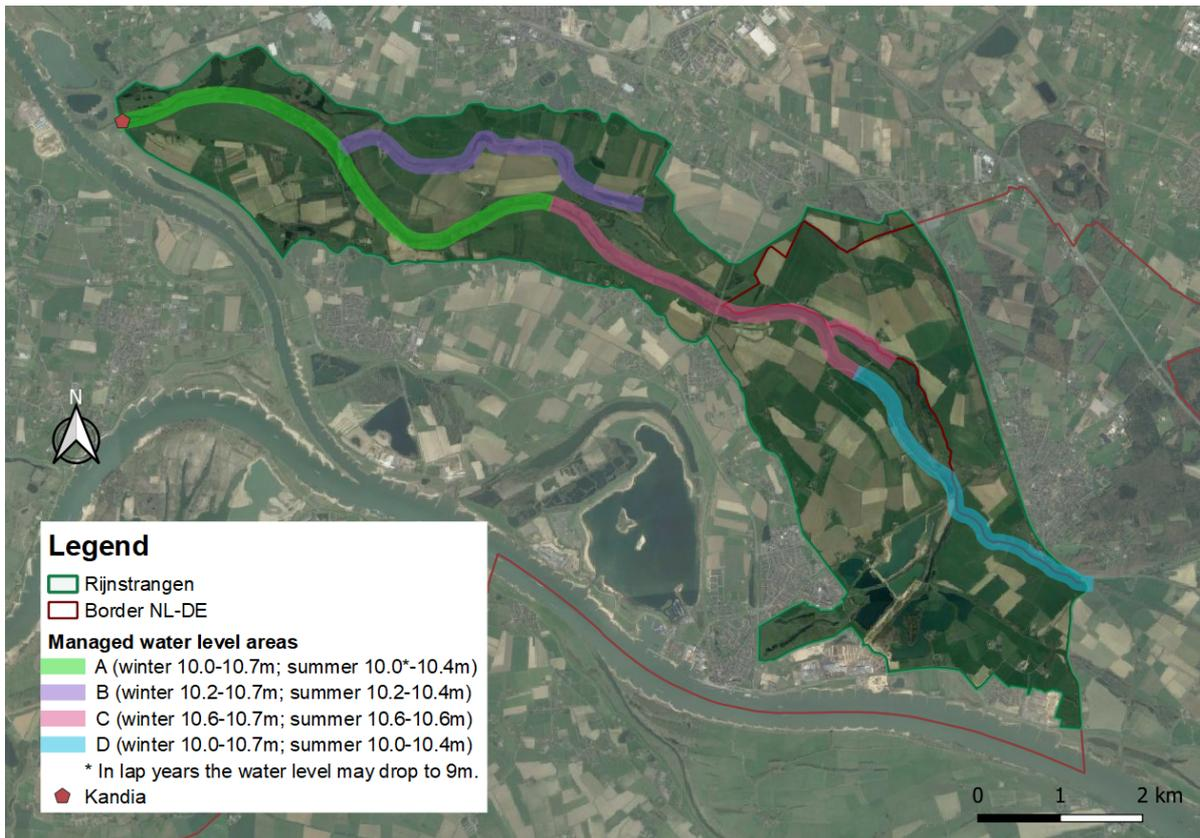
Figure 2.9: Managed water levels in the Rijnstrangen according to the Peilbesluit.
