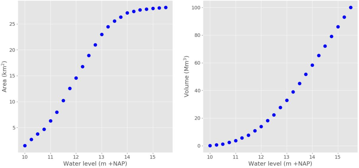
Figure 3.2: Stored volumes of surface water and inundated area for different water levels in the Rijnstrangen.
