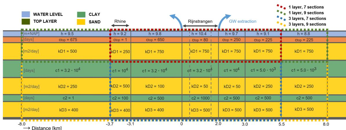
Figure B.1: Schematisation of the geohydrological situation used for the groundwater calculations with extra layers and sections.
