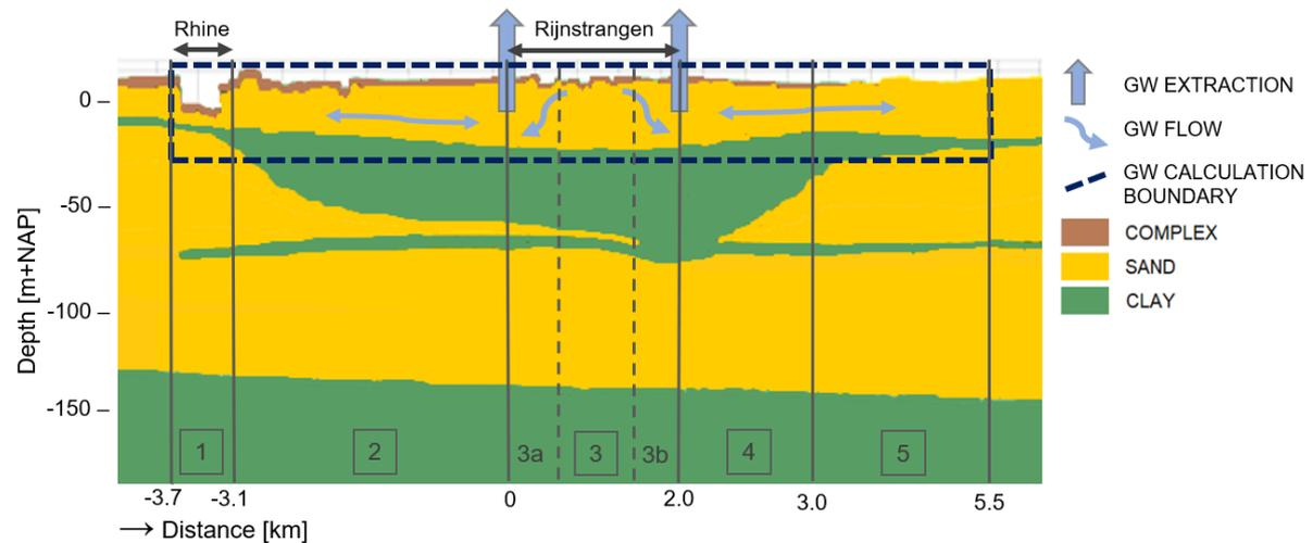
Figure 4.5: Simplified representation of the cross-section for groundwater calculations. The clay layer under the first aquifer is so thick that for this study it acts as the geohydrological base.
