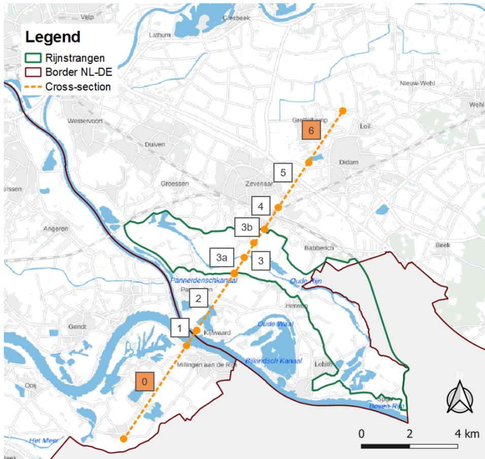
Figure B.2: Map of cross-section for the groundwater calculations, with extra sections. The numbers indicate the different sections as used for the calculation of the groundwater flow. Sections 0 and 6 are not used in the groundwater calculations performed in this study. The effect of these sections on the result of the groundwater calculations is shown in Appendix B.2.
