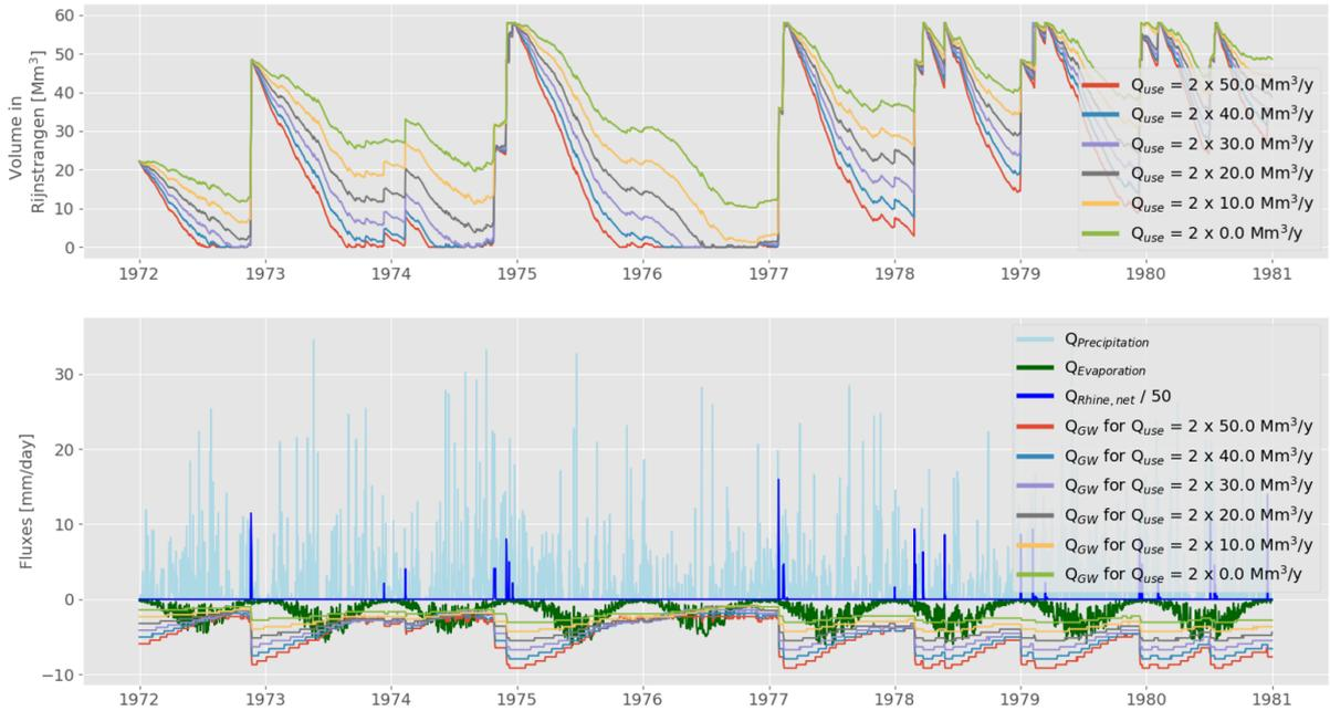
Figure 5.10: Detail of the water balance and corresponding fluxes with the extraction volume ( $Q_{use}$ ) as variable. The river inflow and evaporation are given for the neutral situation.
