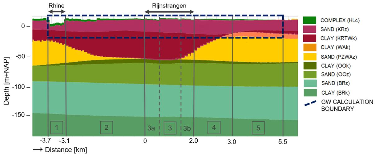
Figure 4.4: Cross-section for the groundwater calculations, as shown on the map in Figure 4.3. It is assumed that this cross-section is representative for the entire Rijnstrangen. The numbers indicate the different sections as used for the calculation of the groundwater flow. Adapted from TNO Geologische Dienst (2021).
