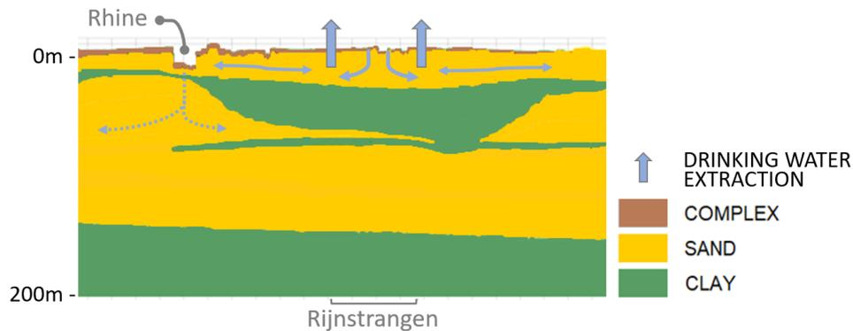
Figure 3.4: Concept of the Rijnstrangen as retention area visualised in a cross-section (indicated in Figure 3.1). The pattern of clay and sand is based on cross-section B - B\* as presented in Figure 2.7, but only indicative.
