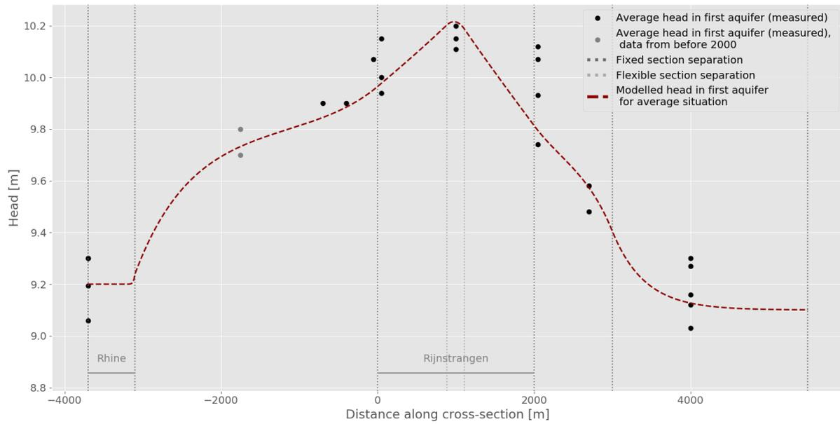
Figure 5.1: Validation of the groundwater model. With a RMSE of 12 cm and from a visual assessment it can be concluded that the groundwater model approximates reality. It is therefore assumed that the values for the groundwater fluxes will be representative as well. Measurement data for heads retrieved from Geologische Dienst Nederland (2021).
