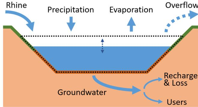
Figure 4.1: Schematisation of the water balance of the Rijnstrangen.
