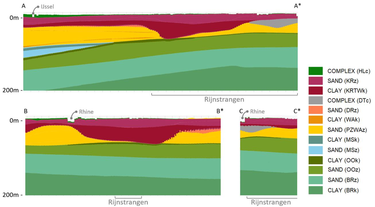
Figure 2.7: Geohydrological situation in the Rijnstrangen region along three cross sections. Adapted from TNO Geologische Dienst (2021).
