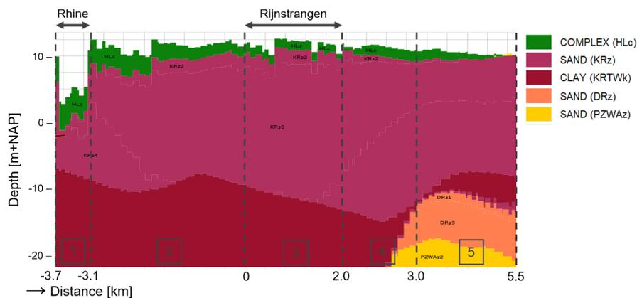
Figure A.2: Cross-section showing the depth of the top layer and the first aquifer. Adapted from TNO Geologische Dienst (2021).
