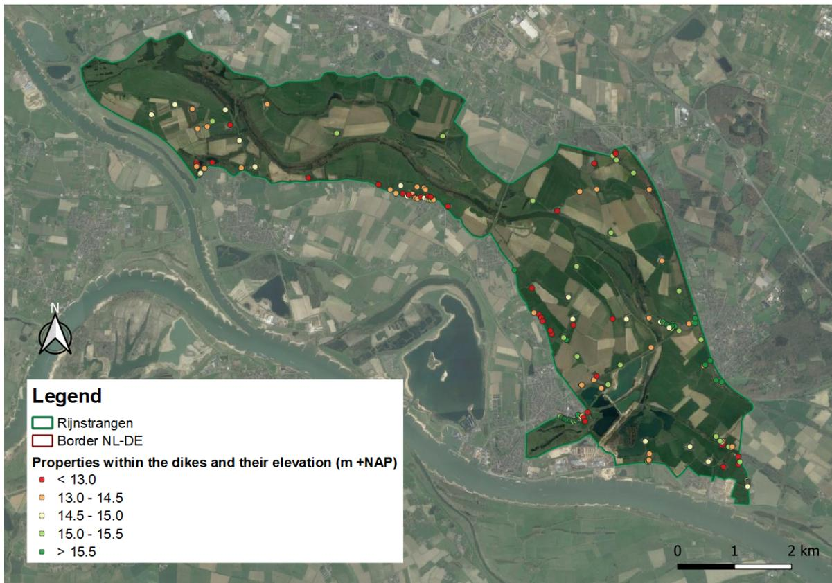
Figure 2.6: Properties within the dikes in the Rijnstrangen and their elevation. The elevation of the properties indicates their safety when flooding the area.
